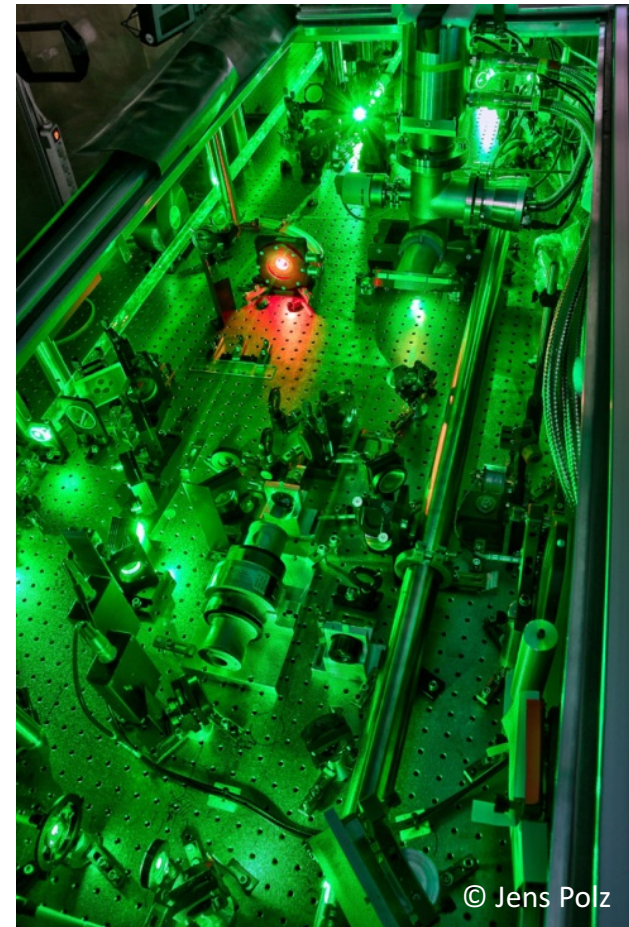
Power amplifier of the JETi laser
